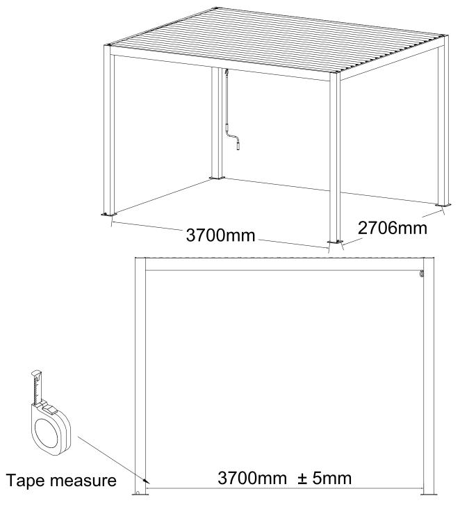
Define installation distance. Measure the distance X at the base of the column, and the difference between the dimension of X and the marked dimension is ± 5mm.
