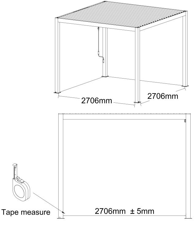
Define installation distance. Measure the distance X at the base of the column, and the difference between the dimension of X and the marked dimension is ± 5mm.
