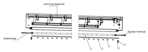
Note: The distance between the cable cards should be 200-250MM.
