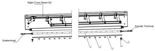
Note: The distance between the cable cards should be 200-250MM.
