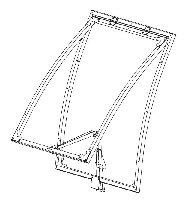
The vent for the greenhouse Strong NOVA is designed to the Greenhouse ventilation and is installed in the roof of the greenhouse with self-tapping screws with a press washer and a rubber seal. Covered with cellular polycarbonate.
