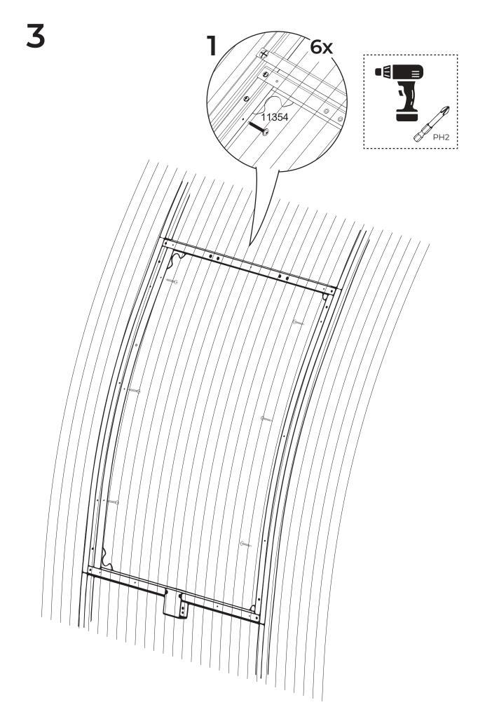
The window frame is mounted from the inside of the greenhouse and the hinges are screwed on from the outside.
