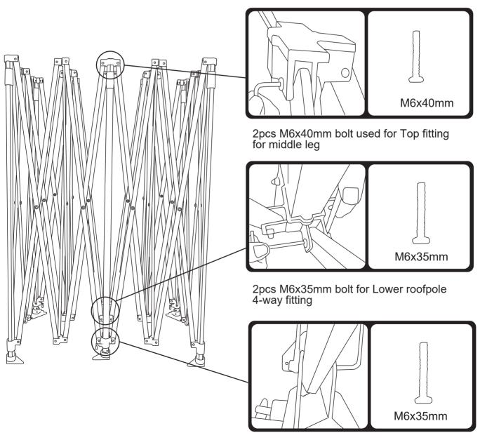
2pcs M6x35mm bolt used for fitting for middle leg
